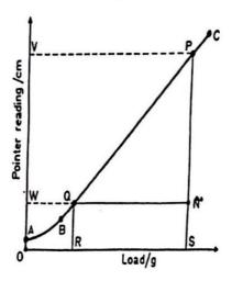
Note. The initial curved portion of the graph is probably due to the fact that in the early stages of the experiment some of the turns of the spring are pressing against each other.
